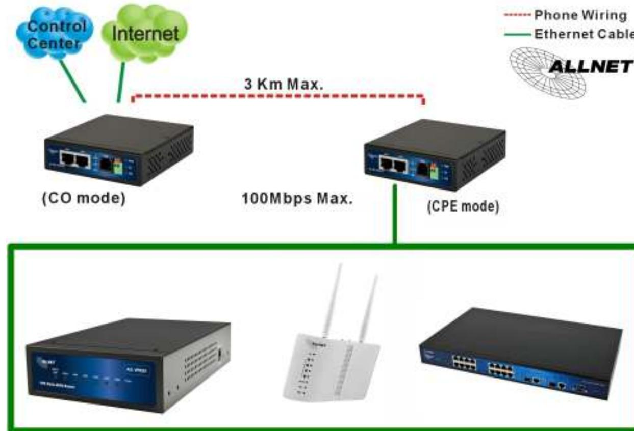
**Figure 2.6 ALL-MC115VDSL2 point to point application diagram**
