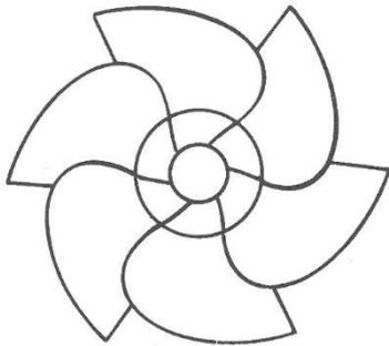
**Fig. 2.** The schematics of an ideal modern sakia, a mechanical water lifting device that used animal power to raise water developed in Nubia (southern Egypt) in the 4<sup>th</sup> century BCE. (P. Fraenkel)
