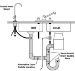
Figure 7: Drain Saddle Assembly Mounting Locations
