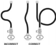
Figure 5: Flexible Hose Positions
