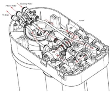
Figure 3: Drinking Water Machine Flow Diagram
