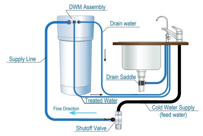
Figure 1: Installation Diagram
