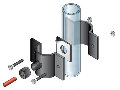
Figure 8: Drain Saddle Assembly
