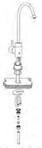
Figure 16: Air Gap Spigot Assembly (Lead Free)\* (treated water spigot)
