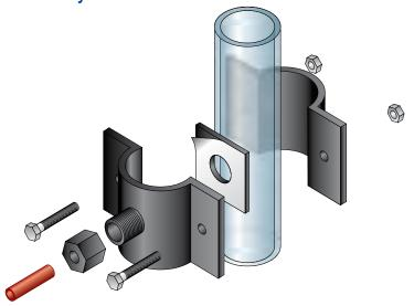
Figure 15: Drain Saddle Assembly
