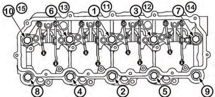
Start installing the bolts with the second bolt from the rear on the top. The hole diameter is smaller, therefore allowing alignment of the remaining bolts.
