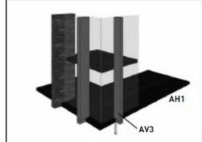
Attach AV6 to AH1 using one (1) screw.
