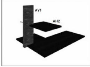
Attach AH2 to AV1 using one [1] screw.
