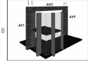
Attach AH3 to AV1 and AV9 using four [4] screws.
