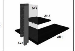
Place AV4 between AH2 and AV2. Attach AV2 to AH2 using one (1) dowel (goes through the hole in AV4). Attach AV2 to AH1 using one (1) screw.
