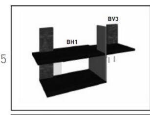
Attach BV3 to BH1 using two (2) screws.
