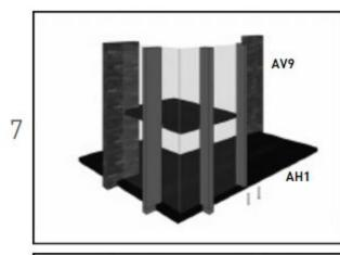
Attach AV9 to AH1 using two (2) screws.
