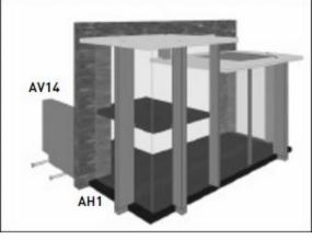
Attach AV14 to AH1 using two (2) screws.
