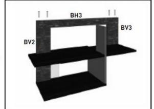
Attach BH3 to BV2 and BV3 using four [4] screws.
