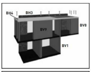
Attach BH4 to BV1, BH3, BV8, BV9 and BV10 using nine (9) screws.
