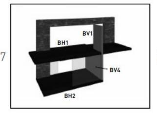
Slide BV4 into place in the grooves in BV1, BH1 and BH2.
