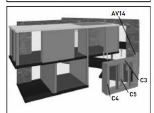
Attach C3 to AV14 using dowel. Attach C4 and C5 to C3 using three (3) screws.
