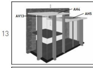
Attach AV13 to AH4 and AH5 using two (2) screws.
