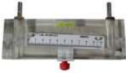
**Definition: Inclined Tube Manometer : Range from 0 - 10 MM WC To 0 - 100 MM WC**
