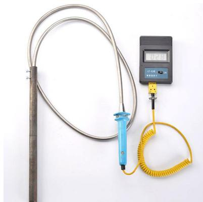
The LT-06 thermometer for liquid aluminum is apply to aluminum processing industry, used to measure the temperature of the liquid aluminum during the smelting procedure. It is consists of type of digital gauge, a probe and a protective sheath. The sheath is installing on the front of the thermometer, it is corrosion resistant to liquid aluminum, can extend the service life of the
