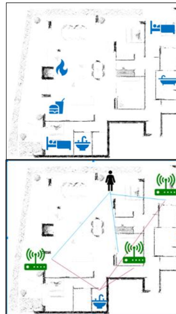
Figure 4: Diagram of original concept implementation which would attempt triangulation to determine localization, this
