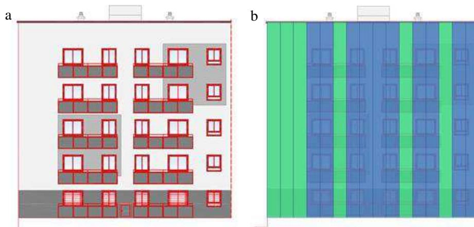
Fig. 1. (a) Target block building located in Madrid; (b) Disposition of panels in the façade.
