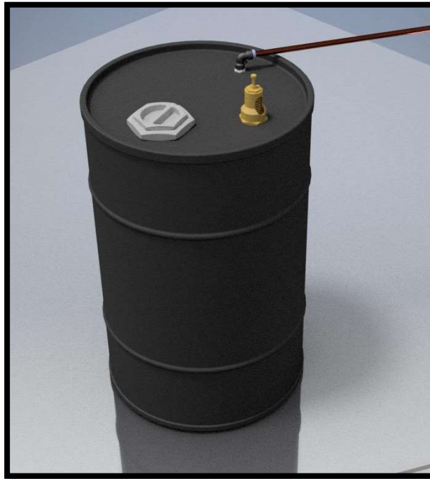
Figure 5.11: Inspection of Pressure Release Valve, Water Input & L Fitting
