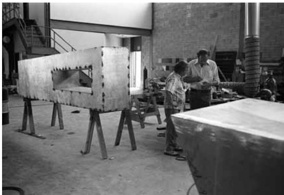
Rosati and Don discussing the components that are tack-welded together prior to a test assembly of the entire sculpture. This is the stage when corrections and adjustments are relatively easy to make, and Rosati is examining the surface flatness, corners, and volumes before work proceeds.
