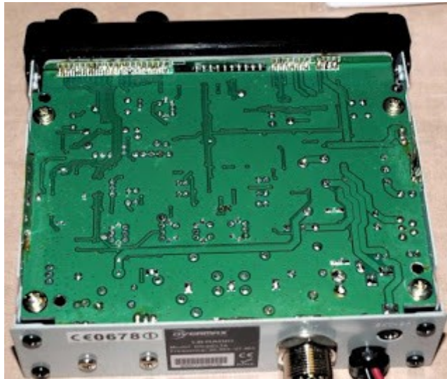
CB-radio OV-DELTA - PCB - góra radia.
