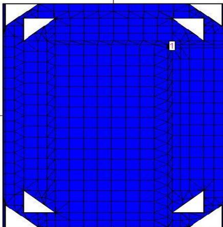
Fig. 3. Second Order Shape of triangularly slotted Sierpinski fractal Antenna
