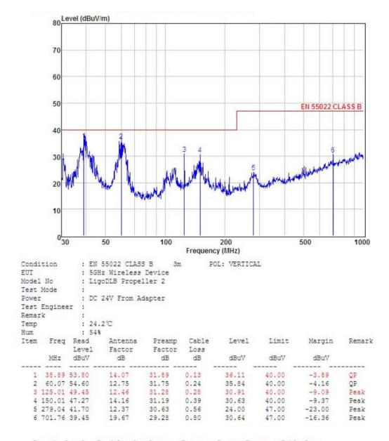
Remark: Level = Read Level + Antenna Factor - Freamp Factor + Cable Loss
