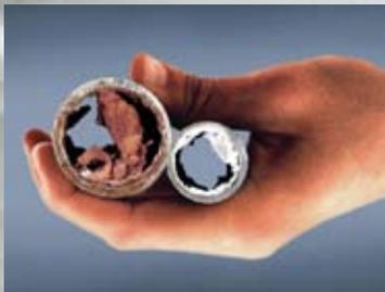
Calcium Scale is a hard thick coating or covering of calcium carbonate ( $\text{CaCO}_3$ ) that forms on heating elements and on the pipes and hardware of plumbing systems. As the calcium rich water enters
