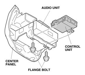
13. Plug the bus cable into the control unit and into the audio unit.
