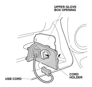
20. With the center panel near the dashboard, plug the USB cord connector into the control unit. Plug in all the vehicle connectors and reinstall the center panel.
