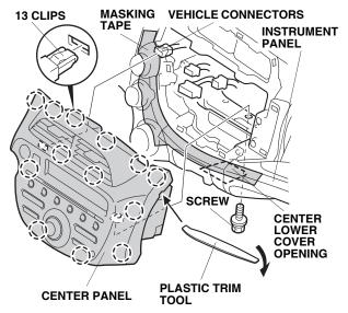
Remove the one screw. Using a plastic trim tool, pull the center panel out toward you to release the 13 clips. Unplug the vehicle connectors to remove the center panel. 10. Get the USB cord. Wrap one urethane tape around the USB cord in the area shown.
