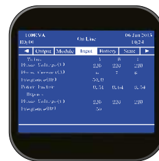
UPS Cabinet Control Panel
