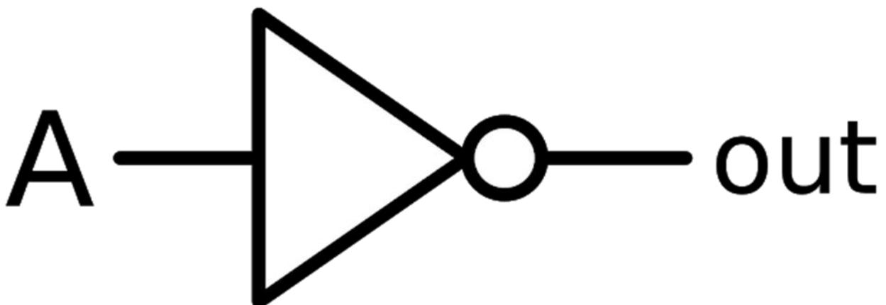
The bubble at the output port represents the inverting operation. That means for high logic signal input, the output of the NOT gate will be LOW, similarly for low logic signal input the output of NOT gate will be HIGH. We can easily understand this by truth table stated below.
