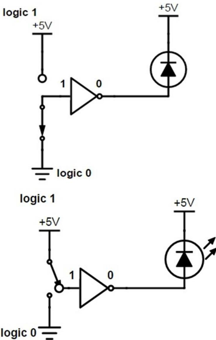
Here we connect an alterable switch with the NOT gate and the output of NOT gate is connected to a LED. An LED is an electronic device which will ON and off when it receives high voltage and low voltage respectively. When the switch is connected to +5 V, the switch is on position so the LED emits light. When the NOT gate is connected to Ground, the LED will OFF so it doesn't emit any light.
