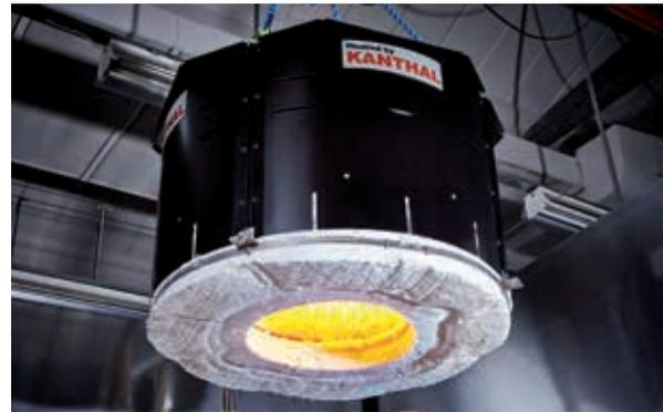
Optionally, certain models can have the heater automatically raised and lowered hydraulically, and there are attachments on both sides to minimize heat loss from the spouts. This goes together with a timer system that starts preheating automatically at a preset time. Heating is monitored and controlled by PLC.
