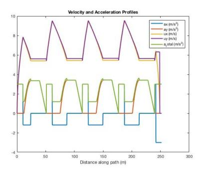
the curvature. Second, we assumed a constant acceleration along each segment of track. Thus, the longitudinal acceleration limit determines the longitudinal velocity, which in turn determines the lateral acceleration based on the total acceleration limit. We then characterized the vehicle's motion as having four discrete regions: accelerating on straightaways, braking into the turn with constant deceleration, holding a constant speed along the turn, and braking just before the finish line.
