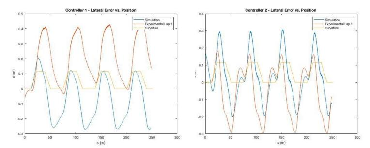
Both controllers seem to exhibit some phase offset relative to our simulation. In the case of Controller 1, there appears to be lag in our controller's responsiveness leading to a 20cm difference in lateral error between simulated and actual results. Our Controller 2 exhibits less phase offset than Controller 1; this is the curvature gain,  $K_k$ , increasing the responsiveness as curvature increases.
