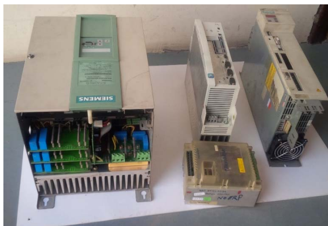
Variable Frequency Drive - VFD
