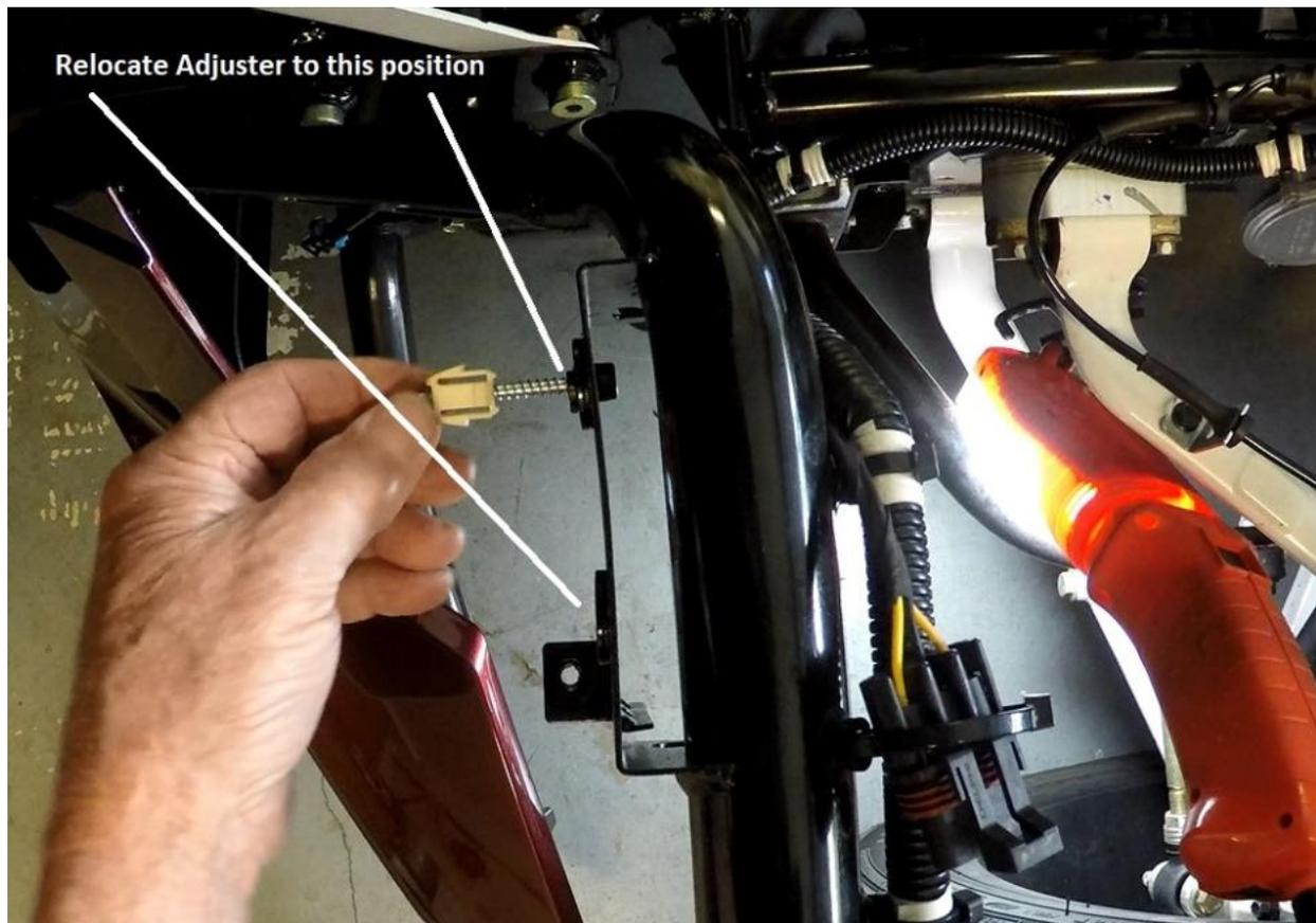
**Step 5:** Remove the 4 mounting screws holding bracket to the stock headlight. Then, with a flat tip screw driver or any flat tool like chisel, pry off the mounting bracket from the stock headlight. There is a rubber grommet and washer in the bracket that will need to be removed for replacement in the new Headlight assembly later.
