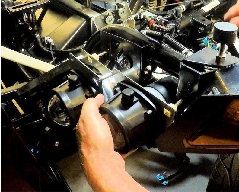
**Step 9:** Remove Side Reflector from Stock Headlight Cover by applying heat from a hair dryer to the reflector front and back to help with removal. Use a chisel to slowly pry up with a slow twisting motion. Heat glue area and then press Reflector firmly into position on New Headlight Cover.
