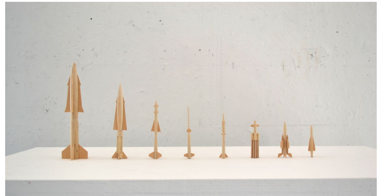
Wooden forms used for casting. These forms were themselves cast into investment media and incinerated in a kiln, leaving voids into which molten bronze was then poured.
