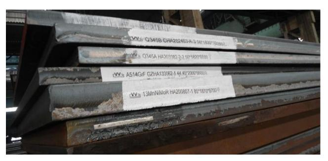
ASTM A514/A514M standard specification covers high-yield, quenched, and tempered alloy steel plates for use in welded parts and other structures. ASTM A514/A514M Standard main steel grade: ASTM A514 Grade A, B, E, F, H, P, Q, S, (A514GRA, A514GRB, A514GRE, A514GRQ, A514GRF, A514GRH) and so on.
