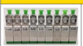
**2.3. SC APC Metal Body** Arvensis Consulting sources their optic fibre attenuators direct from the factory. Our SC/APC attenuators have a  $\geq$ 60dB Return Loss (RL) with the following attenuation accuracy 1-9dB -  $\leq$ 0.5dB 10-30dB -  $\leq$ 10% of the attenuators value Single Mode: 1310nm/1550nm Input Power (Max): 200mW Durability: <0.20dB typical, 1000 mating's Operating temp: -20~+75°C
