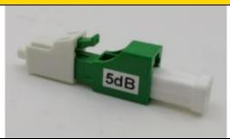
**2.1.LC APC Plastic Body**Arvensis Consulting sources their optic fibre attenuators direct from the<br/>factory. Our LC/APC attenuators have a  $\geq$ 60dB Return Loss (RL) with the<br/>following attenuation accuracy1-9dB -  $\leq$ 0.5dB10-30dB -  $\leq$ 10% of the attenuators valueSingle Mode: 1310nm/1550nm<br/>Input Power (Max): 200mWDurability: <0.20dB typical, 1000 mating's<br/>Operating temp: -20~+75°C
